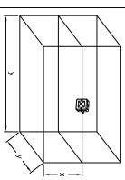
mounting height from the floor and y is the maximum length of the sides of the square floor area covered by the VAD. Wall mounted, where x is the maximum Category W-x-y (Wall mounted):
