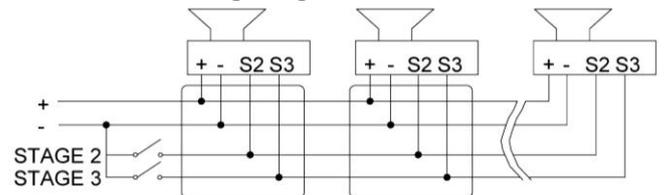
Fig. 5a DC Simplified Block Diagram (negative switching)
