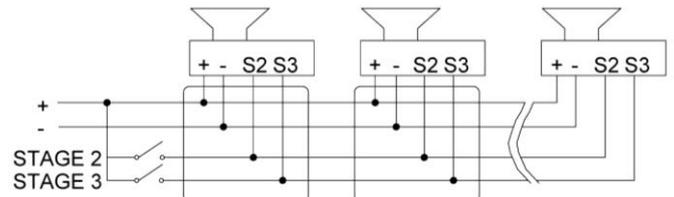
Fig. 5b DC Simplified Block Diagram (positive switching)
